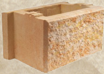
Full Sentinel Wall Block 390mm x 225mm x 200mm 13 per m 2 75 per pallet
