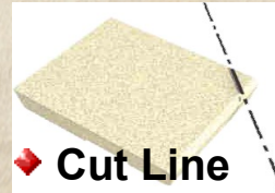
Internal Corner Caps - Cutting Detail
